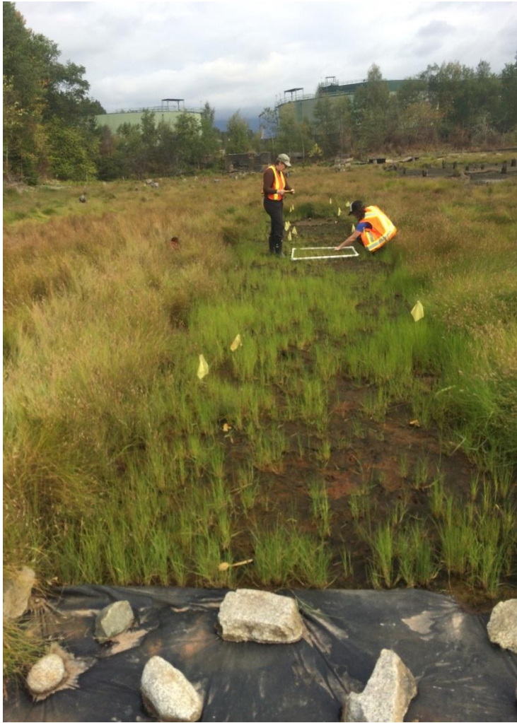
Figure 15. Exposed half of plot (green Spartina plants) previously covered with one layer polyethylene cover in place for one year
